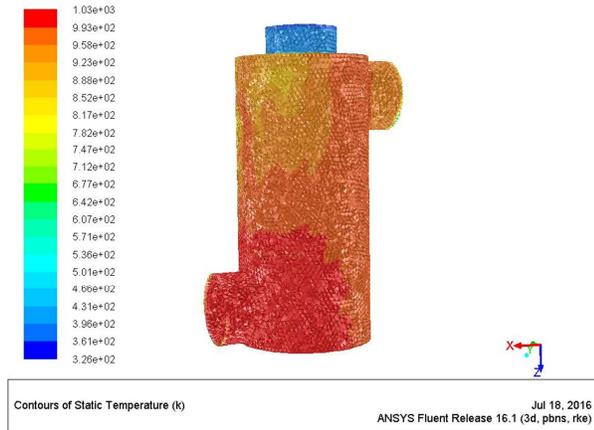
Figure 6. The temperature distribution of the exhaust gas inside the reactor.
