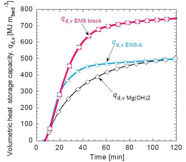
Figure 4. Comparison of volumetric heat storage capacity of pure  $\text{Mg(OH)}_2$ , EM8 in the pellets state and EM8 block [4].
