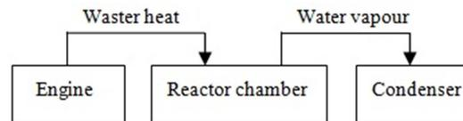
Figure 1. The heat storage process.
