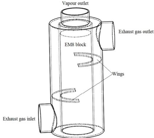
Figure 5. The reactor design.
